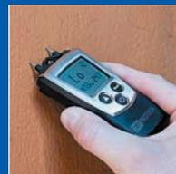
measurement of the wall humidity with the resistance method
